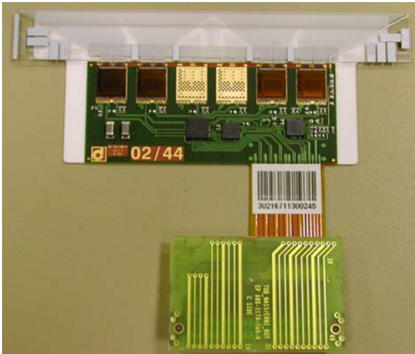
Fig. 6. A front-end read-out hybrid and pitch adapter assembly for the CMS Tracker. The hybrid is produced as a four layer Copper on Kapton circuit, which is then laminated to a ceramic rigidifier prior to component assembly and bonding. The ceramic rigidifier also carries the pitch adapter so that it, together with hybrid, can be integrated into the module as a single assembly. Also shown is an adapter card, which avoids the need for multiple connection cycles on the fragile hybrid connector, during the repeated tests which the hybrid will be subject to prior to its definitive installation in the Tracker
